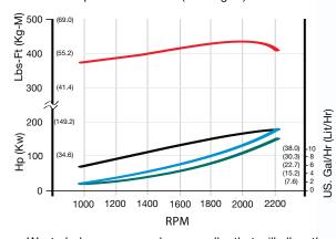
Westerbeke recommends a propeller that will allow the engine to turn 2200 RPM underway at full throttle
