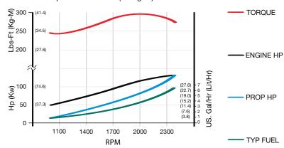
Westerbeke recommends a propeller that will allow the engine to turn 2400 RPM underway at full throttle
